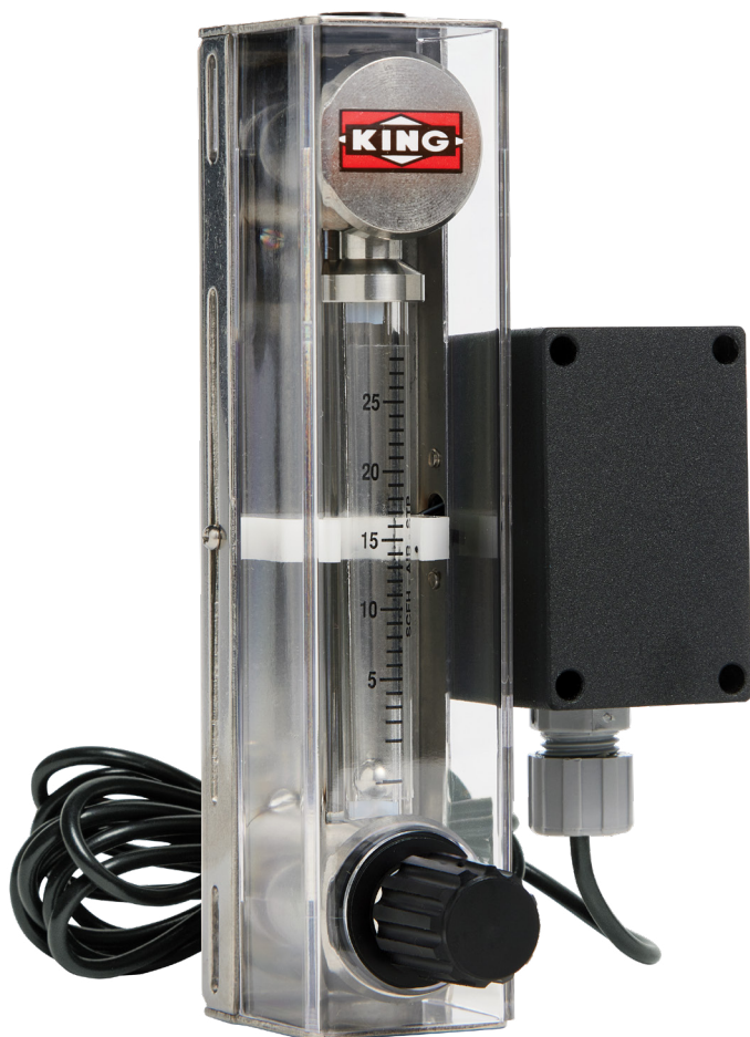
7440 with Fiber Optic Sensor
