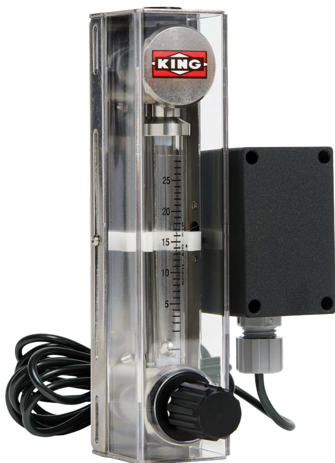
7440 with Fiber Optic Sensor
